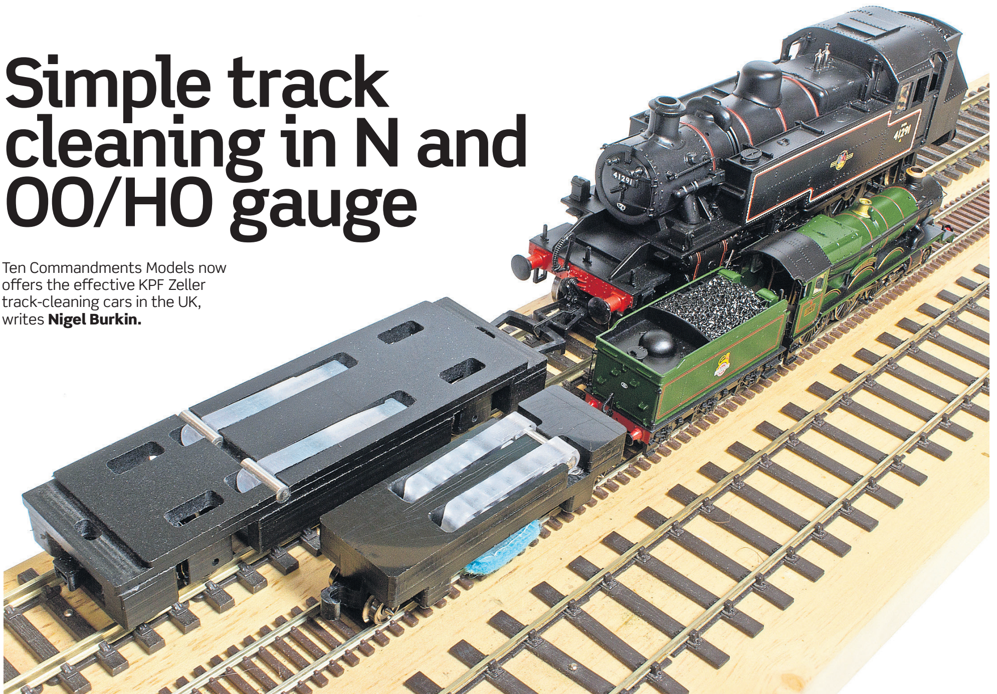
KPF Zeller offers a range of tools for fine tuning and cleaning including a range of rolling roads and track-cleaning cars to suit OO/HO and N gauge track. The cars are sold by Ten Commandments Models in the UK. An O gauge version will become available in the near future.
