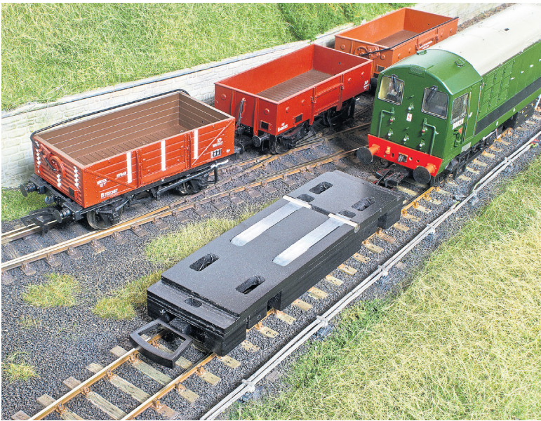
The track-cleaning cars work well when propelled and hauled, which makes them perfect for pushing along end-to-end layouts and working into the end of sidings and platforms.
